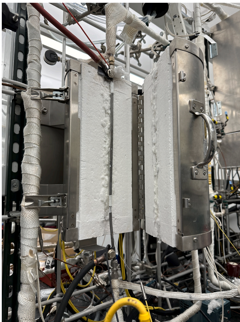
Fig. 4. Reactor tube and insulation furnace.
