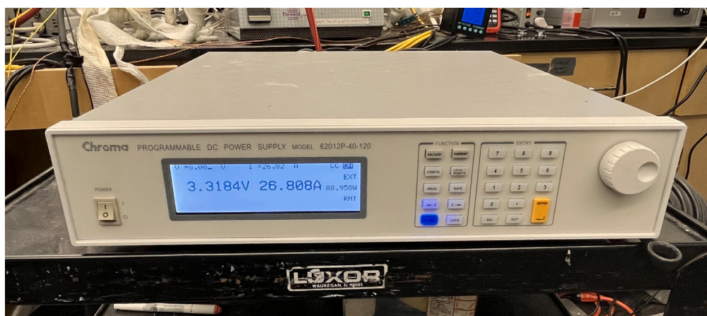
Fig. 5. Power supply connected to the tubular reactor for electrical heating.
