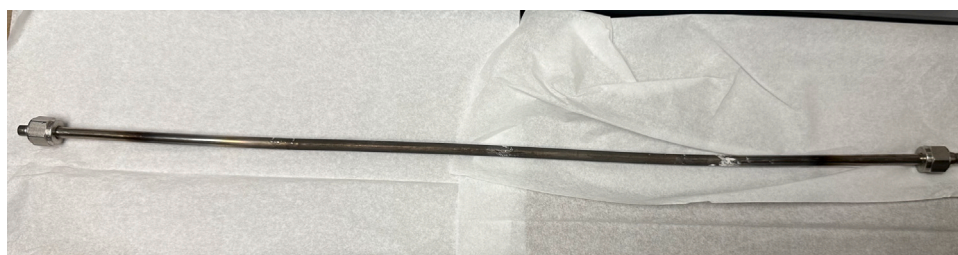
Fig. 4. FeCrAl alloy tube after first oxidation procedure at 950 °C for 10 h.
