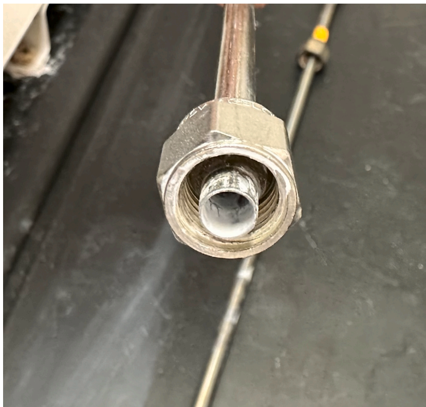
Fig. 6. Wet \text{ZrO}_2 washcoat monolith at the end of FeCrAlloy reformer tube prior to calcination and Ni catalyst embedment.
