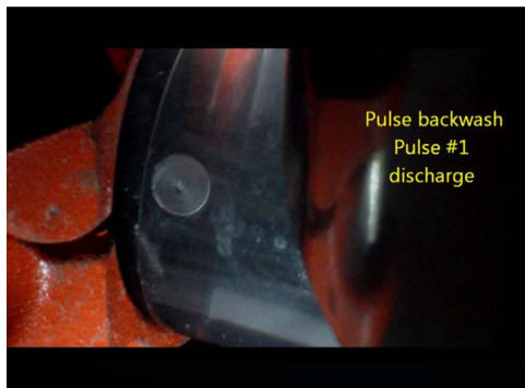
Video 1. Demonstration of UF pulse backwash with RO concentrate during two consecutive accumulator charging and discharging periods. There is a significant release of foulant particles (from the UF elements) which are visible in the transparent section of the drain pipe from the UF module. A video clip is available online. Supplementary material related to this article can be found online at http://dx.doi.org/10.1016/j.memsci.2016.07.022 .
