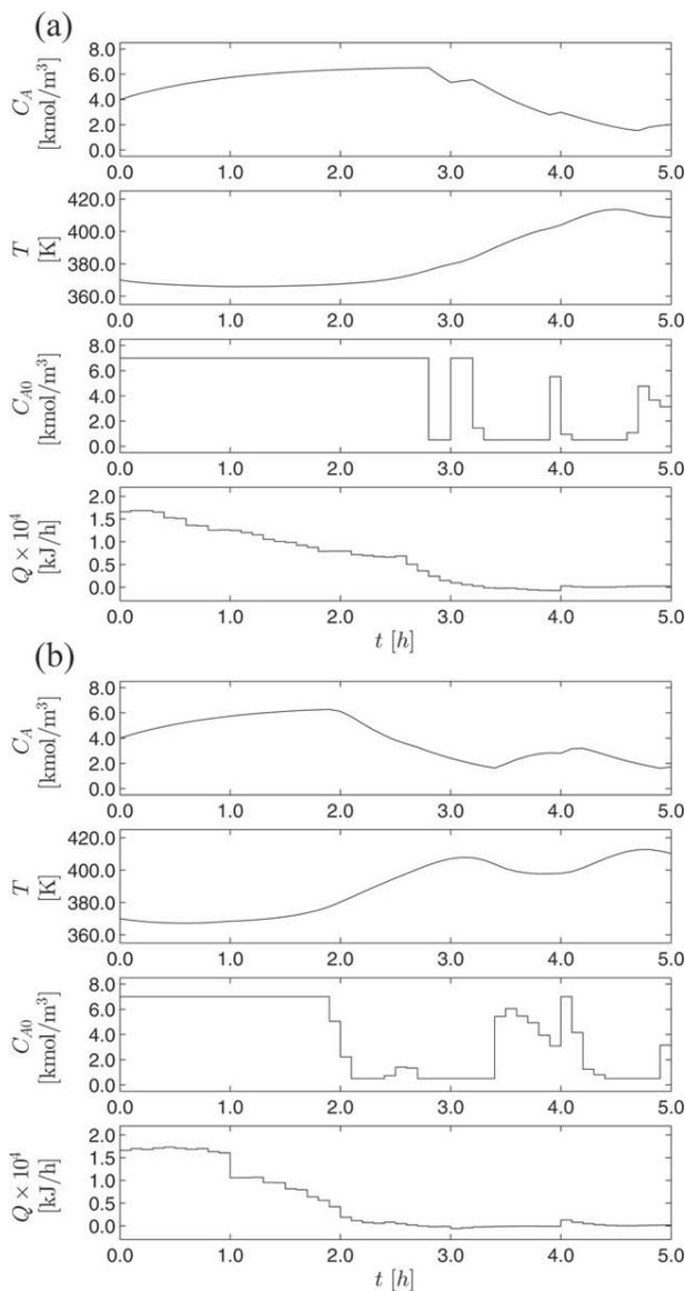
**Figure 7.** The states and inputs of the CSTR under nominal operation with the proposed LEMPC of Eq. 35 initialized at  $C_A(0)=4.0\text{kmol m}^{-3}$  and  $T(0)=370.0\text{K}$  for (a) LEMPC-1 and (b) LEMPC-2.
