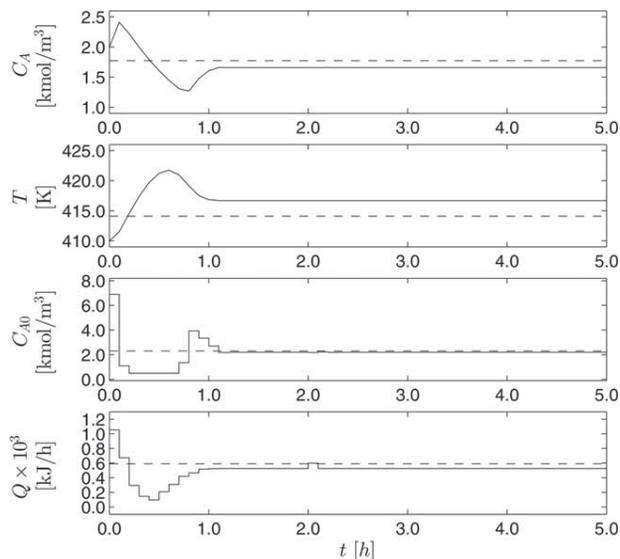
**Figure 5. The states and inputs of the CSTR under the LEMPC of Eq. 35 (i.e., mode 1 operation only) when the economic cost weights are constant with time (solid line) with the economically optimal steady state (dashed line).**
