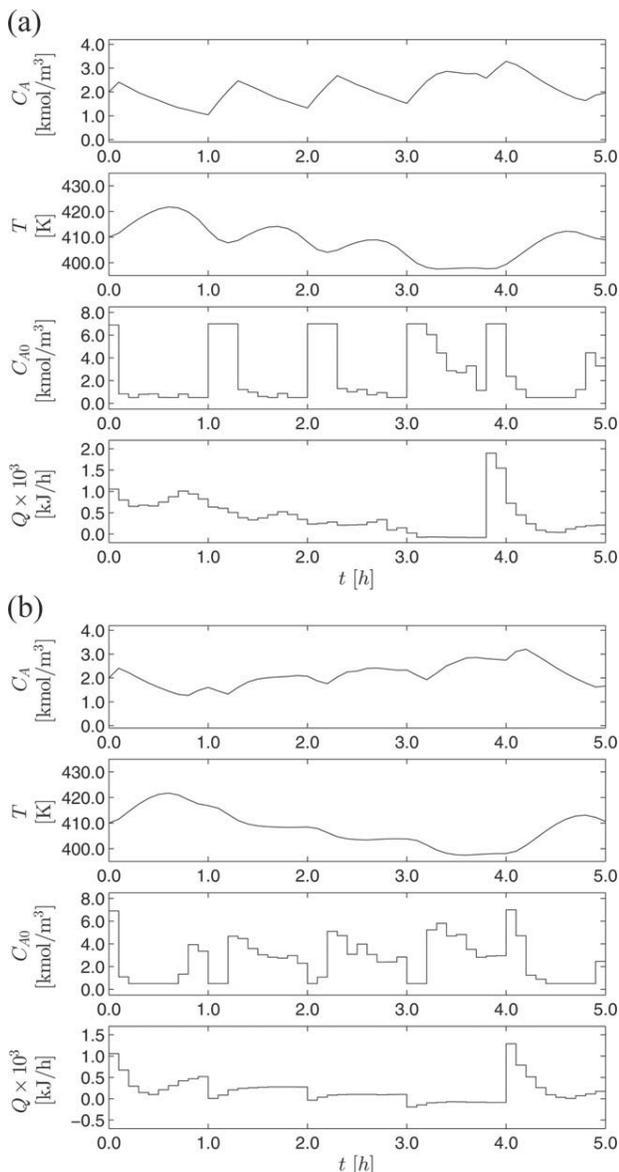
**Figure 4. The states and inputs of the CSTR under nominal operation with the proposed LEMPC of Eq. 35 (i.e., mode 1 operation only) initialized at  $C_A(0)=2.0\text{kmol m}^{-3}$  and  $T(0)=410.0\text{K}$  for (a) LEMPC-1 and (b) LEMPC-2.**
