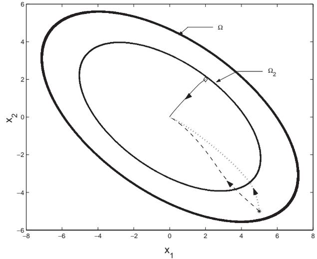
Fig. 6. Closed-loop state trajectory starting close to the origin using MPC with  $T = 1.2$  (solid) and from a point farther away in state space using the switching scheme with a horizon length  $T = 1.2$  (dotted) and using only MPC with  $T = 1.5$  (dashed).
