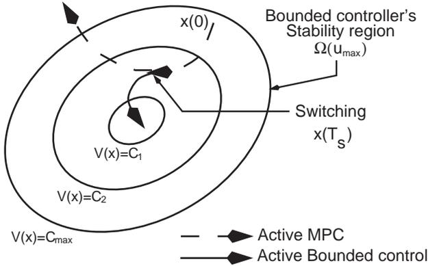
Fig. 2. A schematic representation of the implementation of the stability-based switching scheme of Theorem 1.
