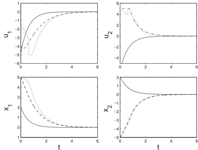
Fig. 7. Input and closed-loop state profiles starting close to the origin using MPC with  $T = 1.2$  (solid) and from a point farther away in state space using the switching scheme with a horizon length  $T = 1.2$  (dotted) and using only MPC with  $T = 1.5$  (dashed).
