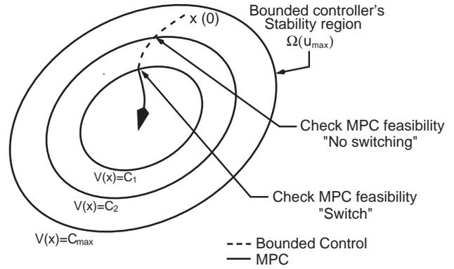
Fig. 3. A schematic representation of feasibility-based switching using a stability-handling MPC formulation.
