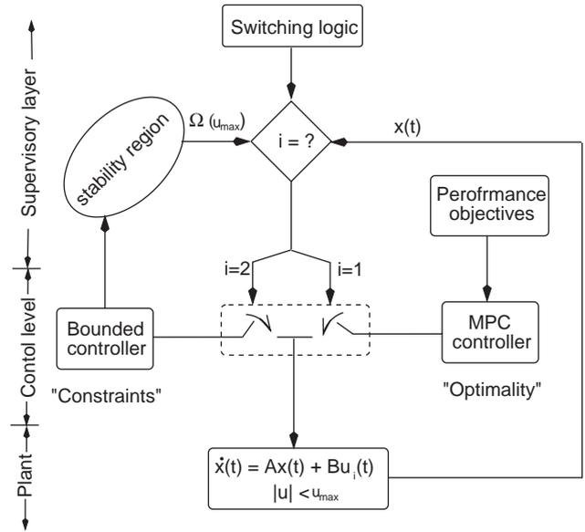
Fig. 1. A schematic representation of the hierarchical hybrid control structure merging the bounded and MPC controllers.
