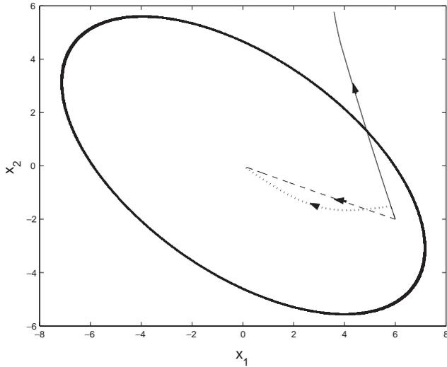
Fig. 4. Closed-loop state trajectory under MPC with  $T = 1$  (solid), under the switching scheme of Theorem 1 with  $T = 1$  (dotted), and under MPC with  $T = 1.5$  (dashed).
