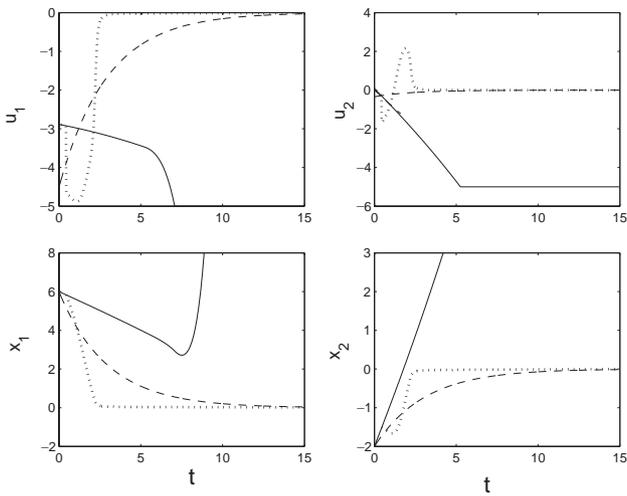
Fig. 5. Input and closed-loop state profiles under MPC with  $T = 1$  (solid), under the switching scheme of Theorem 1 with  $T = 1$  (dotted), and under MPC with  $T = 1.5$  (dashed).
