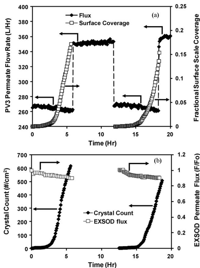
**Fig. 5.** Demonstration of BWRO plant operation in normal feed flow and feed flow reversal (Run 3, Table 3). (a) Permeate flow from PV3 of the BWRO plant and fractional area coverage by scale in the EXSOD membrane test section. (b) Crystal number density in the EXSOD membrane test section and total permeate flux for the EXSOD monitor. Initial gypsum saturation was 2.37 and 2.0 at the BWRO membrane surface of PV3 and the EXSOD membrane test section, respectively.
