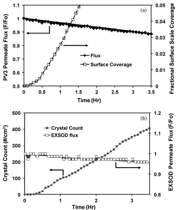
**Fig. 4.** Demonstration of BWRO plant operation in normal feed flow mode (Run 2, Table 3). (a) Permeate flow from PV3 of the BWRO plant and fractional area coverage by scale in the EXSOD membrane test section. (b) Crystal number density in the EXSOD membrane test section and total permeate flux for the EXSOD monitor. Initial gypsum saturation was 2.9 and 2.57 at the BWRO membrane surface of PV3 and the EXSOD membrane test section, respectively (Table 3).
