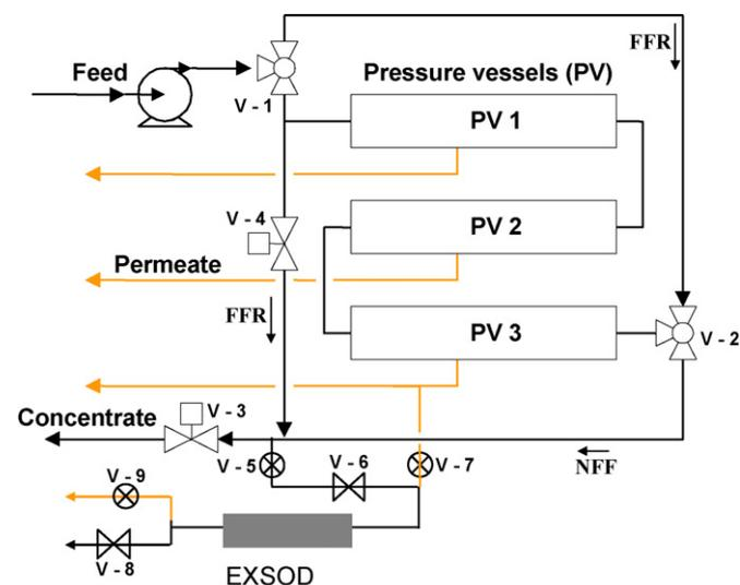
**Fig. 2.** Flow reversal manifold with the EXSOD monitor mounted on the concentrate stream with computer controlled valves to switch between the concentrate and permeate side streams as alternate feeds to the EXSOD monitor. NFF and FFR indicate normal direction and reverse feed flow direction, respectively, with the arrows indicating the corresponding flow directions.
