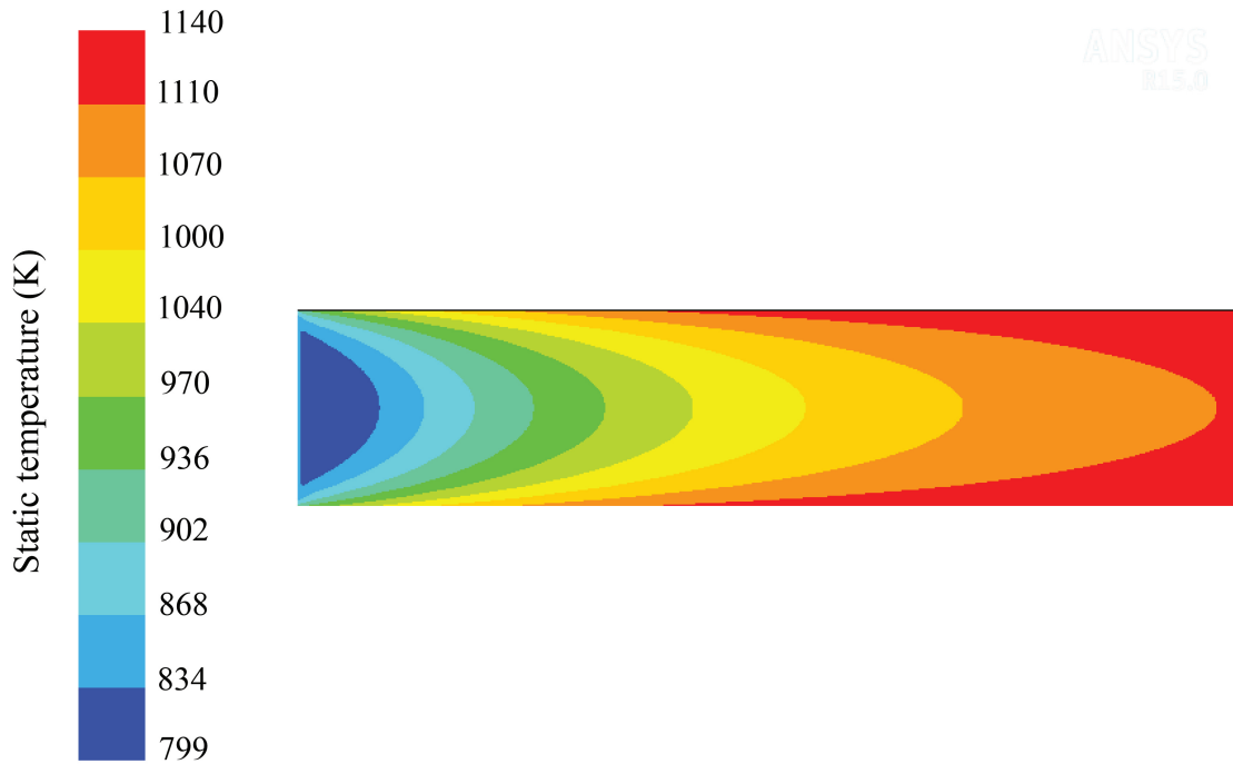
Figure 2.4: Temperature profile from the reforming tube CFD simulation, where the outer reforming tube wall temperature profile (Fig. 2.3(a)) is that fitted based on the available SMR plant data. 38
