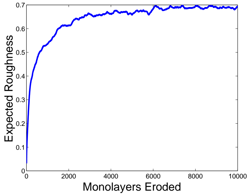
Figure 3.7: Profiles of the expected open-loop surface roughness of the sputtering process.
