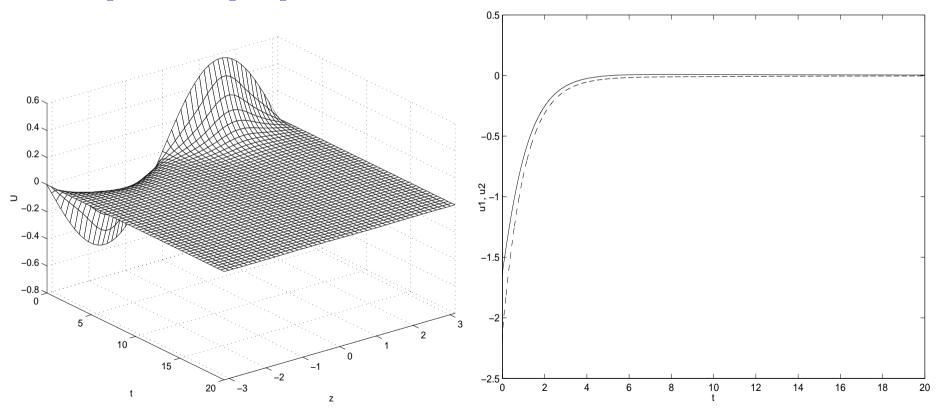
• Profiles of KSE under output feedback control, for the optimal actuator/sensor locations, for  $x_s(0) = [0 \ \phi_2]$  and uncertainty in  $\nu$ . Manipulated input profiles - Solid line  $u_1$  and dashed line  $u_2$
